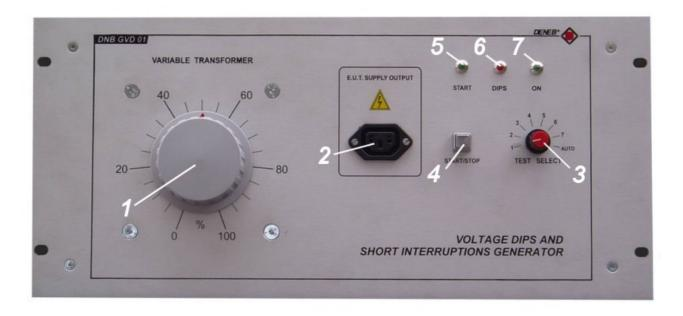
1 - VARIAC, necessary to set up in precise way the level of test previewed from the norm and relative dip. For example if we set the variac to the level of test 0% we have set up a dip of the 100% because a dip is a voltage fall from max (100%) until the level of the variac, while if we set the variac at level test of 40% we have set up a dip of 60%. The norms previews to set up the Variac to 3 level tests: 0, 40 and 70%.
